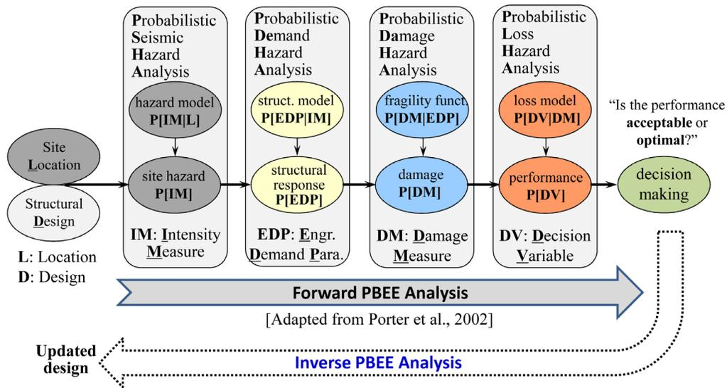
**Figure 1:** Forward PBEE analysis and need for inverse PBEE analysis
